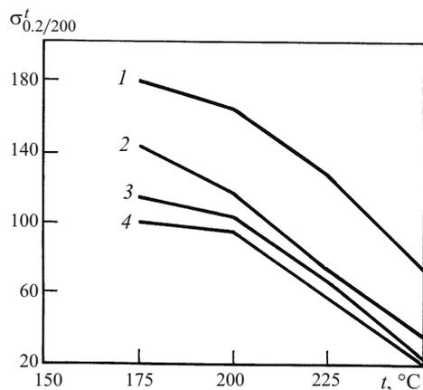
**Fig. 4.** Dependence of the creep resistance  $\sigma_{0.2/200}^t$  (the stress ensuring a creep strain of 0.2% after a 200-h hold at an elevated temperature) on the test temperature of alloys: 1) MRI201S-T6; 2) MRI202S-T6; 3) MRI206S-T6; 4) A319-T6.
