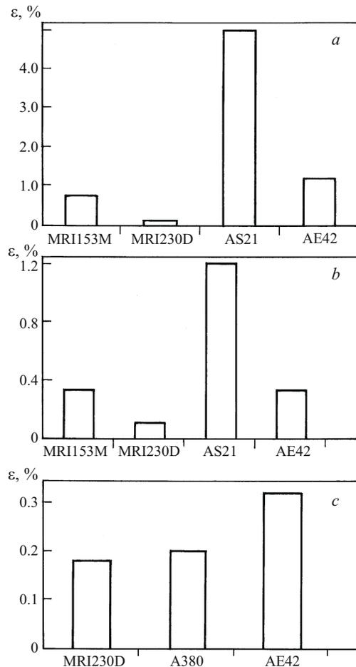
**Fig. 3.** Creep strain  $\varepsilon$  of magnesium alloys MEI153M and MRI230D, commercial alloys AS21 and AE42, and aluminum alloy A380. The test for creep strength lasted for 200 h: a) at a temperature  $t = 135^\circ\text{C}$  and a stress  $\sigma = 100 \text{ MPa}$ ; b)  $t = 150^\circ\text{C}$ ,  $\sigma = 70 \text{ MPa}$ ; c)  $t = 175^\circ\text{C}$ ,  $\sigma = 70 \text{ MPa}$ .
