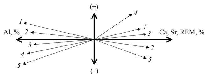
Fig. 2. Diagram reflecting the effect of Al, Ca, Sr, and REM on the properties and cost of magnesium alloys for high-pressure die casting: 1) strength at room temperature; 2) casting properties; 3) cost; 4) creep resistance; 5) ductility, impact toughness.
